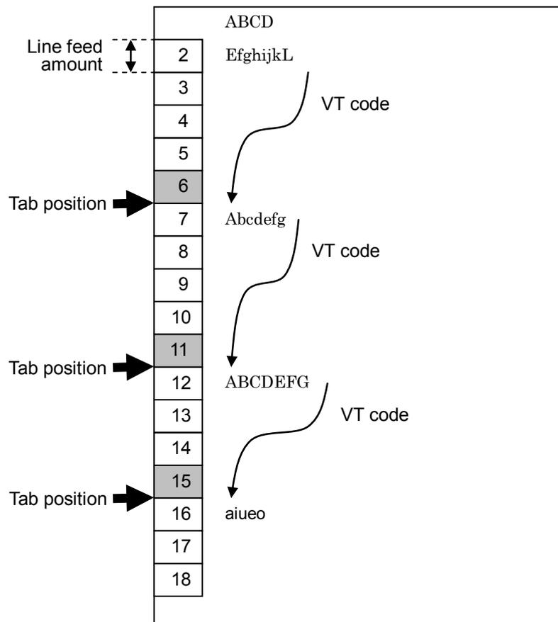
Example: Vertical tabs are specified at Lines 6, 11, and 15, and data is entered while VT are performed.
