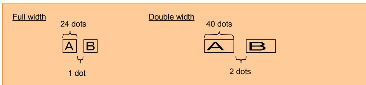
**ESC g    Apply micron pitch**
