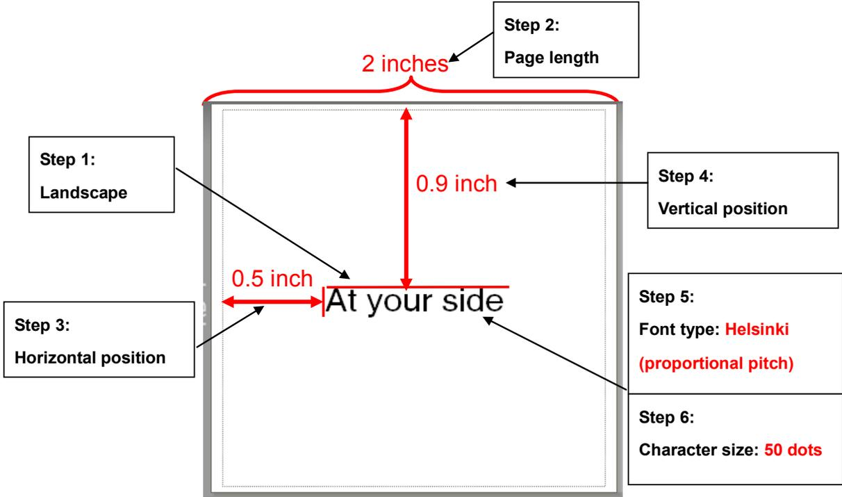
In order to make this label, the following six steps are required after entering ESC/P mode.
