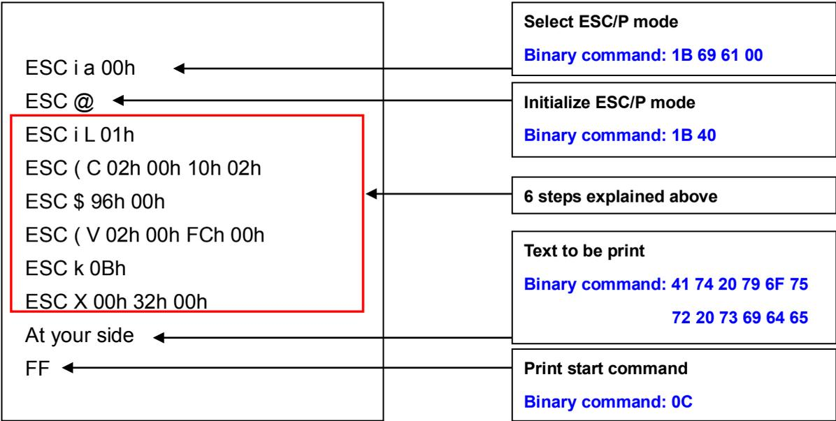
However, these commands should be converted to binary data before sent to the printer, as shown below. Here is the captured converted binary data.
