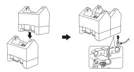
Connect one end of the included DC cord to the DC connector OUT of the first battery charger and connect the other end of the DC cord to the DC connector IN of the second battery charger.
