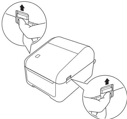
3. Hold the printer by the front, and firmly lift the Roll Compartment Cover to open it.
