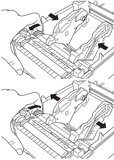
5. Insert the roll so that the label print side is facing up, as shown in the illustration.
