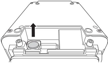
5. Insert the new battery into the battery slot, making sure the battery is level and its positive side is facing up.
