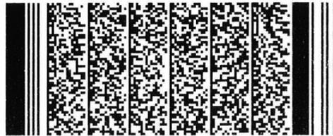
Data compression method: P1 Error correction level: E4 Center pattern in barcode area: M1 Human Readable: Yes: U50,300,50 Module Width 4 dots: W4 Bar Height 4 dots: H4 Maximum Number of Rows: 60 Rows: R60 Maximum number of columns: 4 Cols: C4 Truncation:1: T0 Expression length:297: L297
