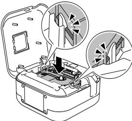
4. Press the Tape Cassette into the label printer until it snaps into place and close the cover.
