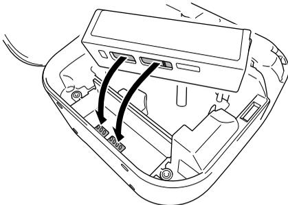
5. When reinserting the battery, make sure the battery's contacts are touching the contacts inside the battery compartment.
