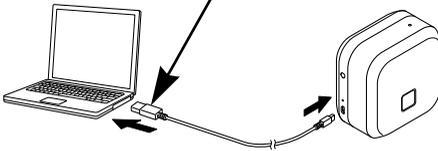
2. Connect the label printer to the computer using the included USB cable, or connect the USB cable to a USB AC Adapter suitable for charging mobile devices and plug the adapter into a power source. Charge until the Battery LED turns off.
