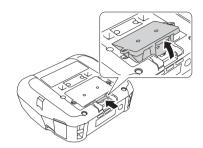
2 Insert the Dummy Battery Pack assembly until it locks into place.
