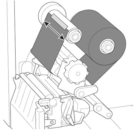
6. Wind the Ribbon Rewind Spindle counterclockwise about three to five turns until the ribbon is smooth, flat and without wrinkles.
