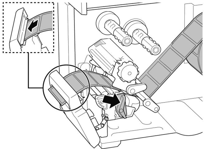
6. Move the Media Sensor by adjusting the Media Sensor Position Adjustment Knob. Make sure the position of the Gap or Black Mark Sensor matches the position of the Gap/Black Mark on the label roll.
