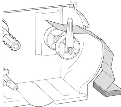
3. Push the Print Head Release Lever and thread the label through the Damper, Media Sensor, and Front Label Guide to install the media.
