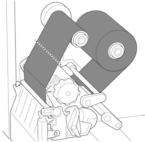
2. Remove the ribbon from the Ribbon Rewind Spindle.
