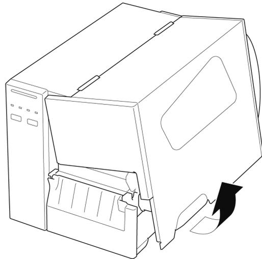
2. Slide the Label Roll Guard horizontally to the end of the Label Supply Spindle, and then flip down the Label Roll Guard.
