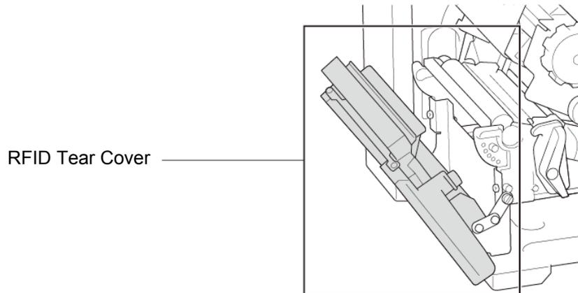
3. Feed the RFID media through the Tear Cover Slot.
