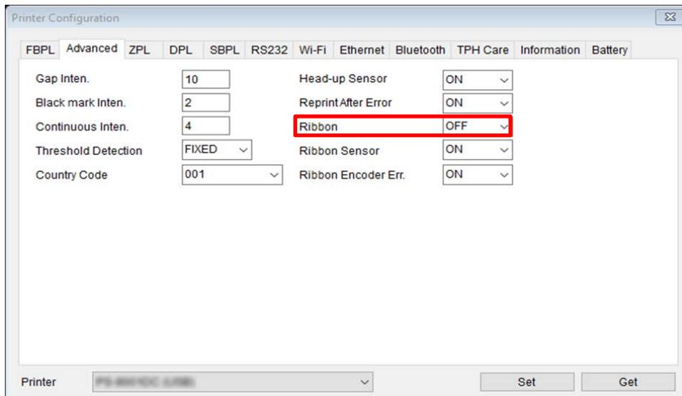
**When setting the Thermal Transfer method:**
