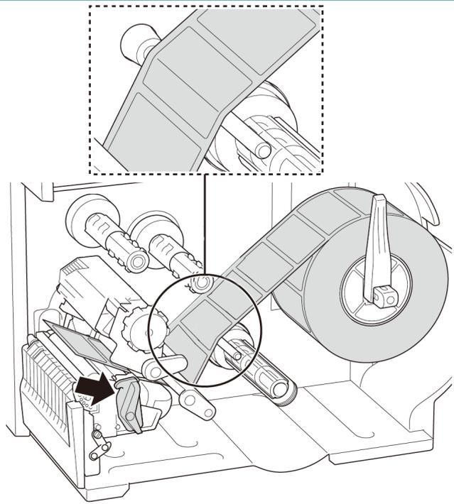
5. Move the Media Sensor by adjusting the Media Sensor Position Adjustment Knob. Make sure the position of the Gap or Black Mark Sensor matches the position of the Gap/Black Mark on the label roll.
