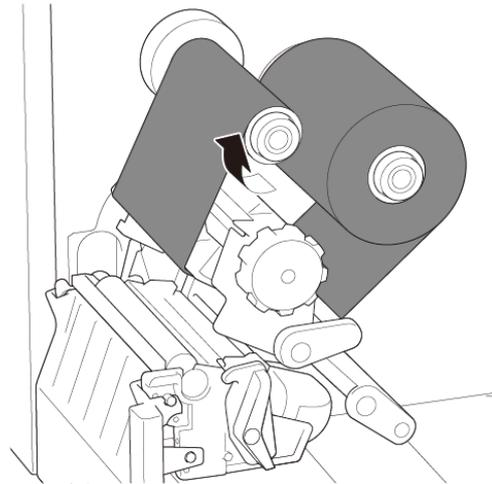
7. Close the Print Head by pushing down on both sides of the Print Head Release Lever.
