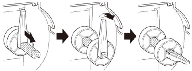
3. Place the label roll on the Label Supply Spindle and then flip the Label Roll Guard upwards to hold it in place.
