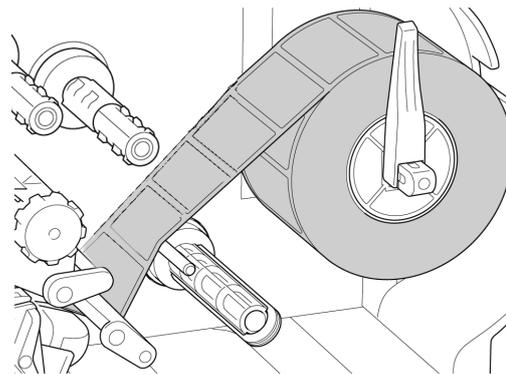
10. Turn the Print Head Release Lever, and pull approximately 650 mm of the label roll through the Media Output Slot.
