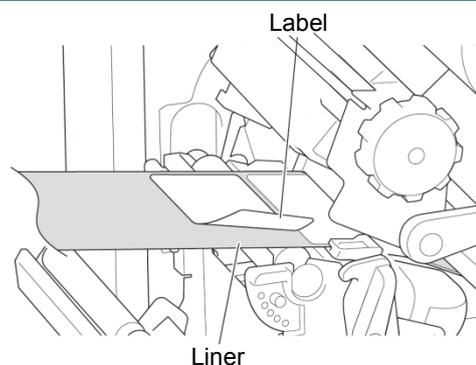
12. Thread the liner through the Label Peeler Cover Slot.
