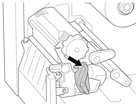
4. Thread the ribbon under the ribbon guide bar and through the ribbon sensor slot following the loading path printed on the Label Printer Cover.
