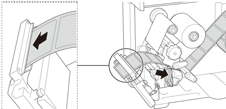
4. Move the media sensor by adjusting the Media Sensor Position Adjustment Knob. Make sure the position of the Gap or Black Mark Sensor matches the position of the Gap/Black Mark on the label roll.
