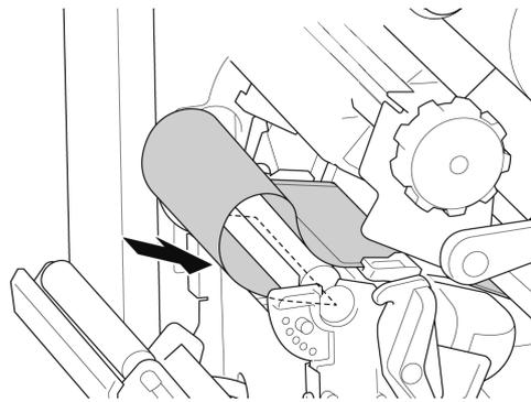
13. Pull the Liner Securing Clip out from the Liner Rewind Spindle, and wind the liner on the Liner Rewind Spindle until the liner is fully stretched.
