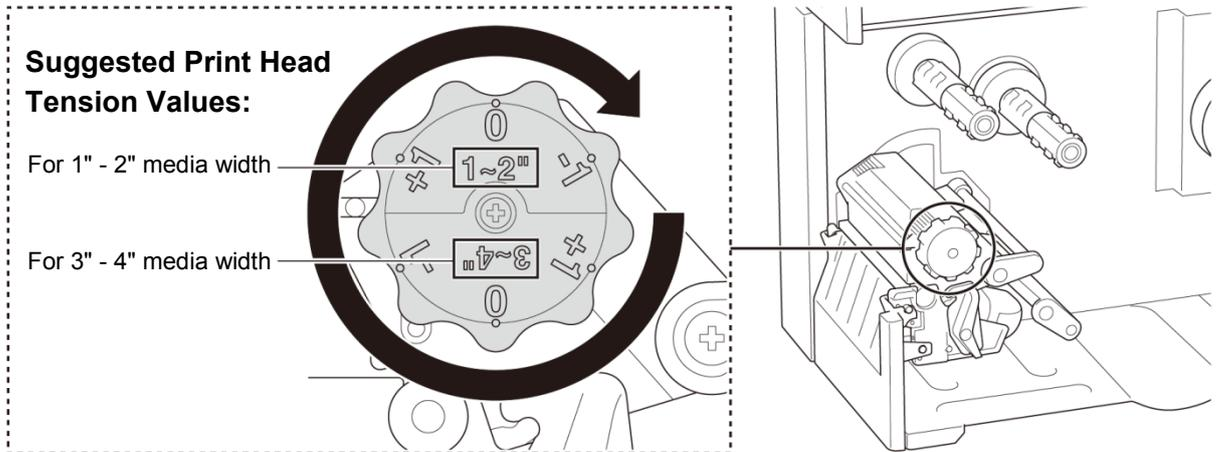
For the best print quality, adjust the Print Head using the Print Head Tension Adjustment Knob. Choose one of six levels of tension adjustment depending on the media width you use (1" - 2" or 3" - 4").
