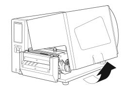
3. Slide the Label Roll Guard horizontally to the end of the Label Supply Spindle, and then flip down the Label Roll Guard.
